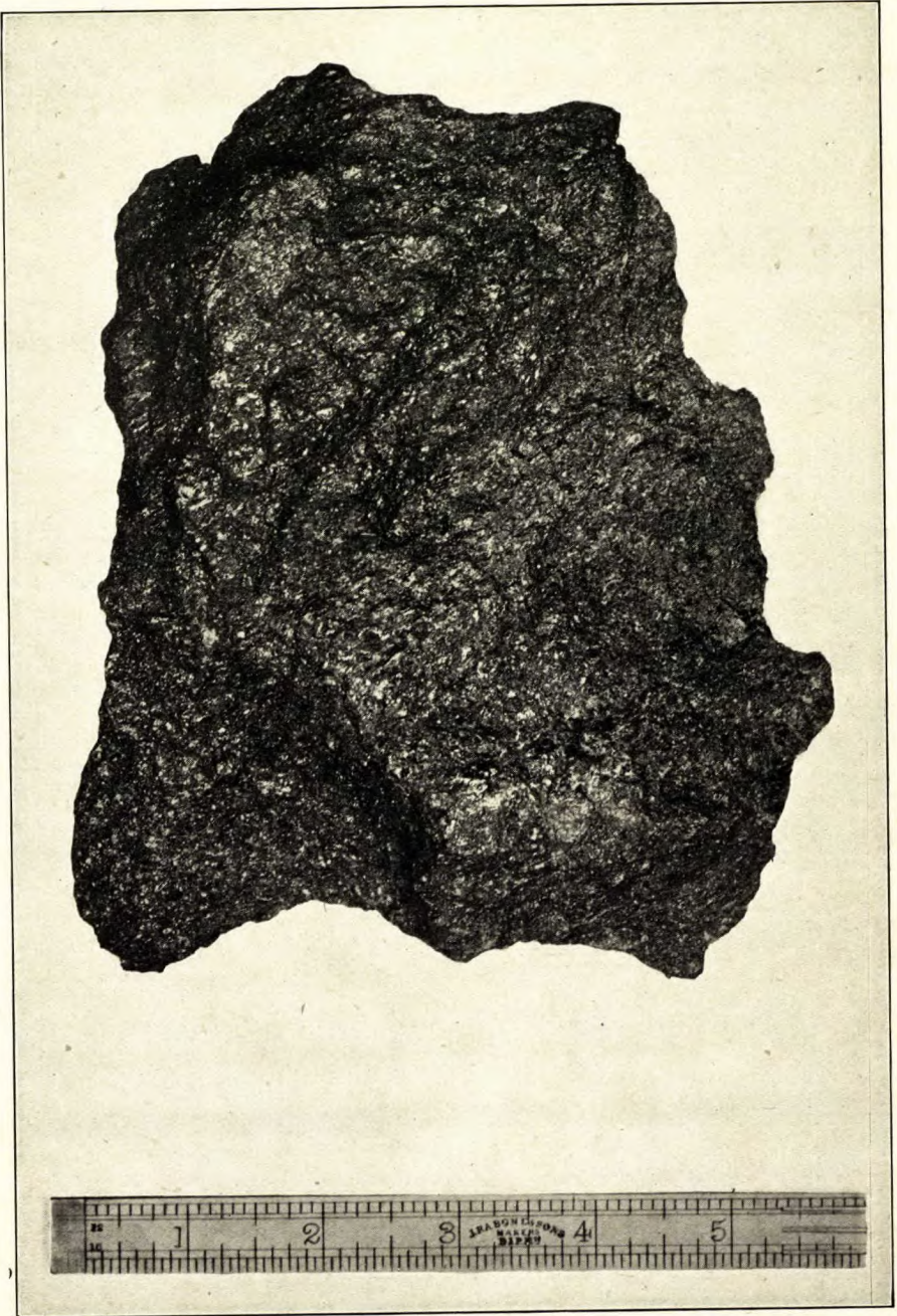
Typical high grade, Canadian flake graphite ore, 15-20 per cent carbon, from the Buckingham district, Que.
