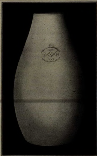
Type of retort, used in the smelting of gold, silver, zinc, etc. (Joseph Dixon Crucible Company, Jersey City, N.J.)
