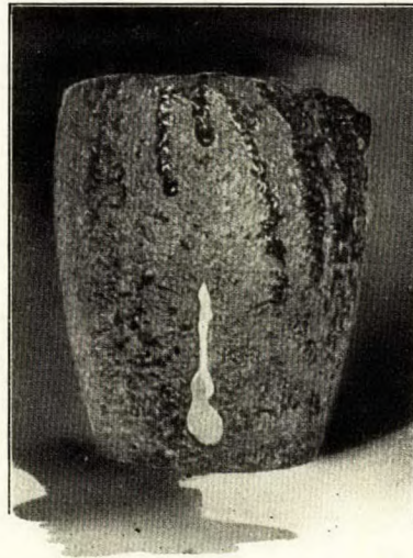
PIN HOLE OR LEAK
