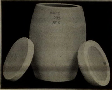
Type of crucible used in melting steel. (Joseph Dixon Crucible Company, Jersey City, N.J.)
