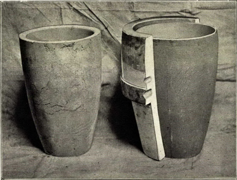
Crucibles as removed from the moulds. (Crossley Machine Company, Trenton, N.J.)
