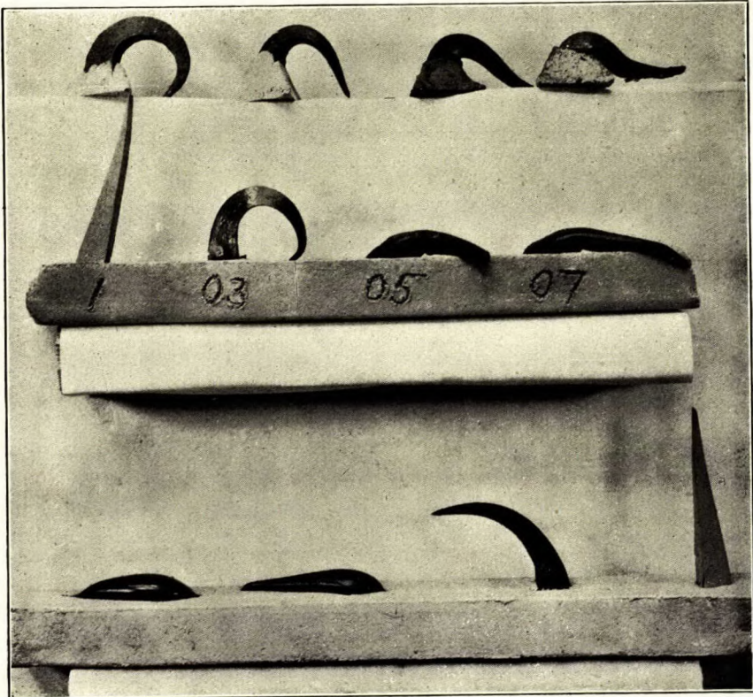
Top row, clay test cones. Middle row } standard seger cones. Bottom row }
