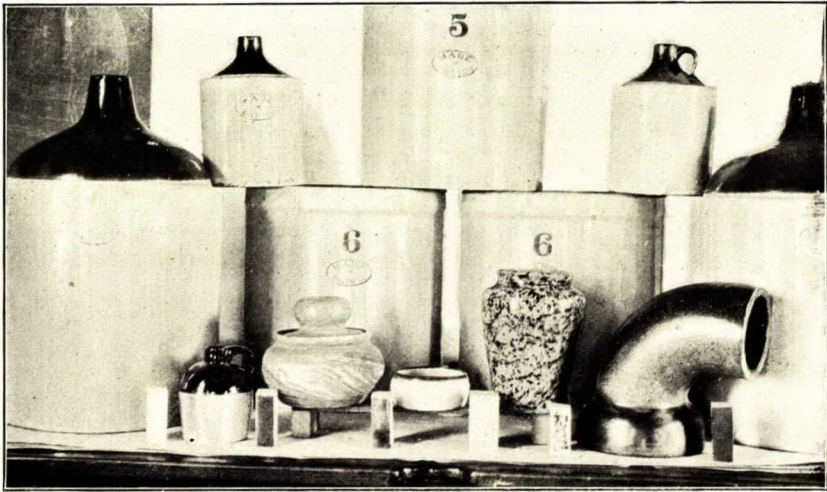
Stoneware pottery and sewerpipe, made from Eastend clays illustrated on Plate VI.
