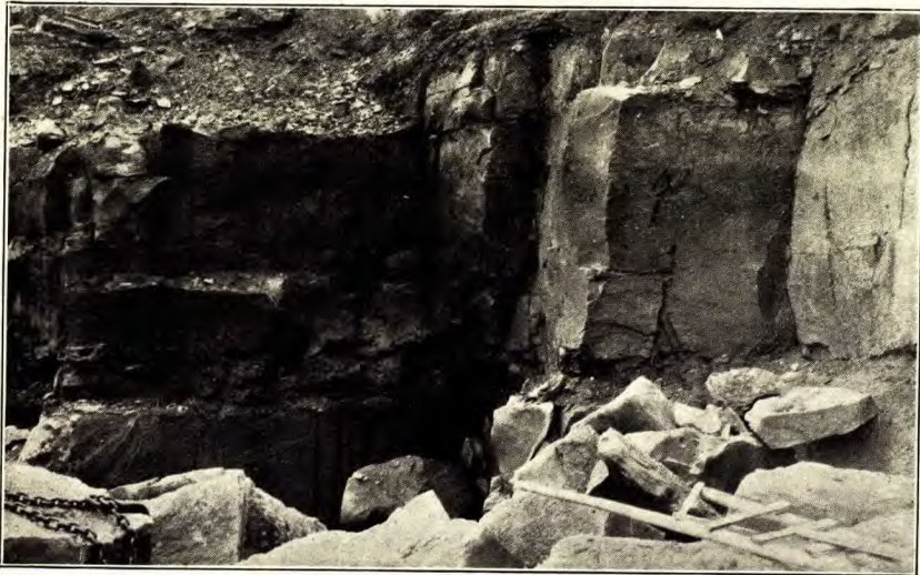
Lower beds, Miramichi Quarry Co., Limited, Quarryville, N.B. (These beds of sandstone are from 10 to 12 feet in thickness.)
