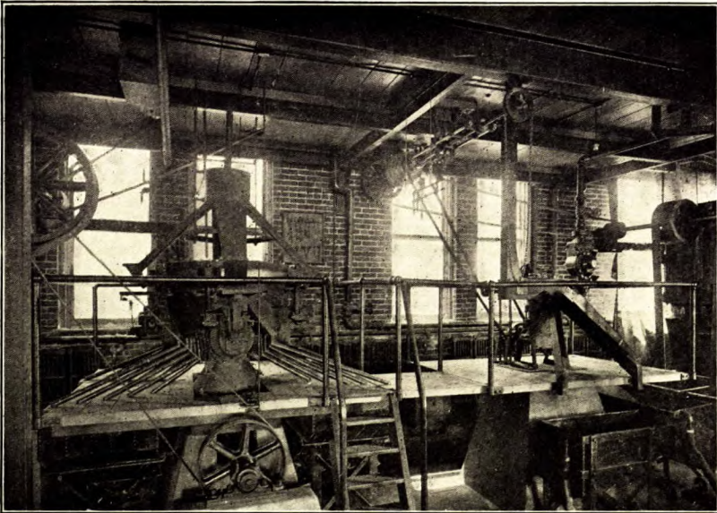
Ore dressing laboratory: Ulrich magnetic separator, left; Richards pulsator jig, right.
