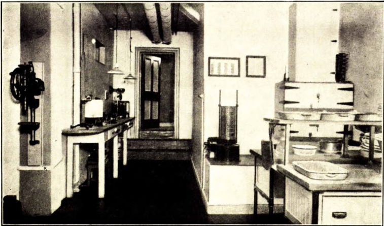
Structural materials laboratory: mixing table, sieve agitator, moist closet, and asphalt testing apparatus
