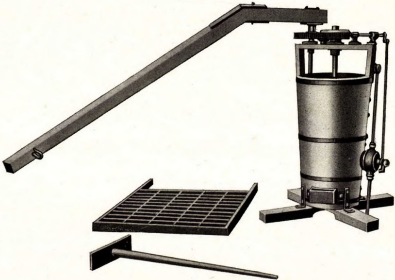
Egeberg peat pulping machine operated by horse-power.
