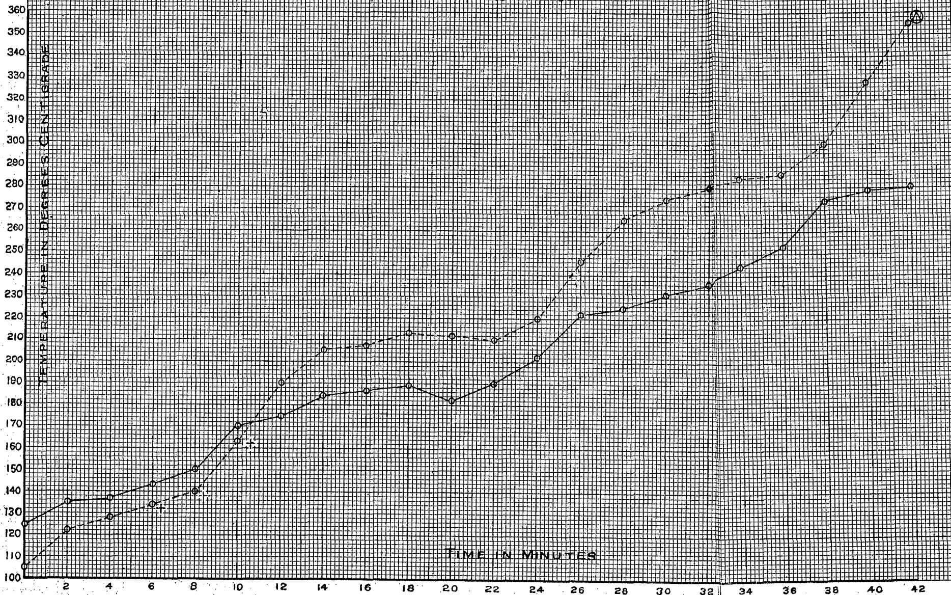
FIG. 51. Absorption of oxygen by powdered Carterville coal in air (15).
