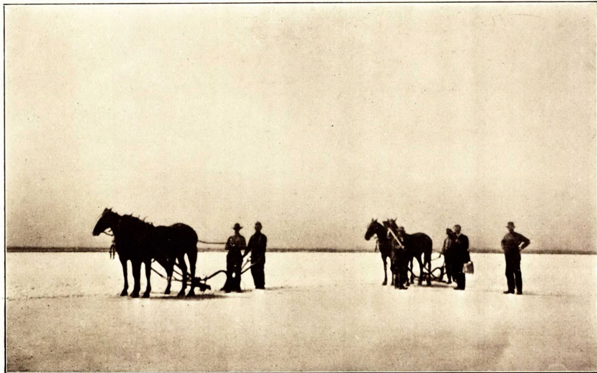
Ploughing salt in harvesting pond, Inland Crystal Salt Co., Saltair, shore of Great Salt lake, near Salt Lake City, Utah.
