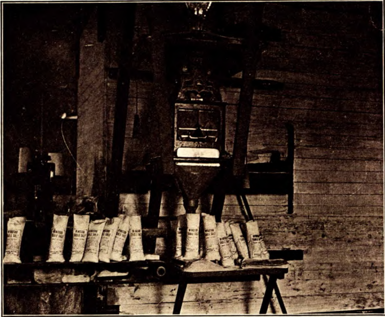
A. Automatic bagging machine and bag sewer, Canadian Salt Co., Windsor, Ont.
