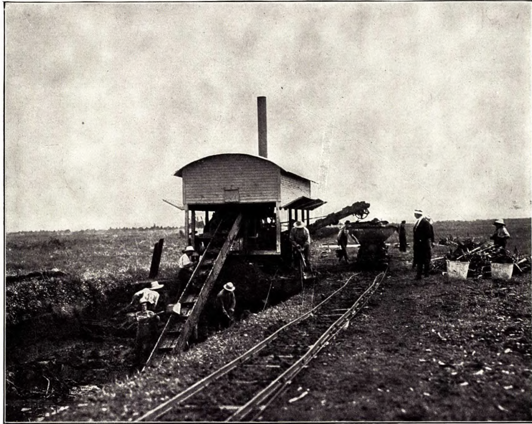
30 ton Anrep peat machine: end elevation, showing elevator, trenching operations, and track.
