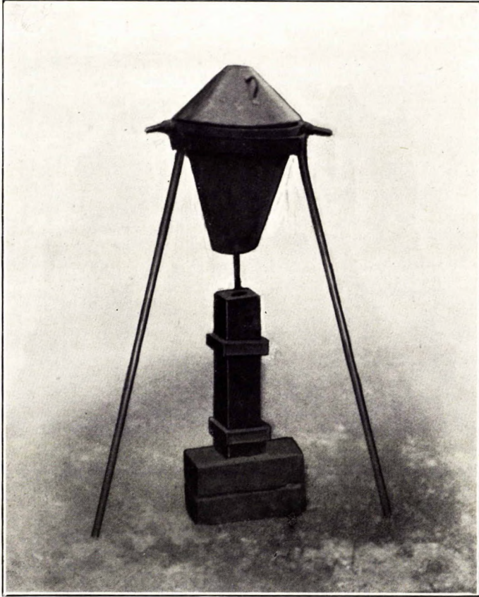
Crucible for the reduction of \text{Co}_2\text{O}_3 with Al: in position over mould.
