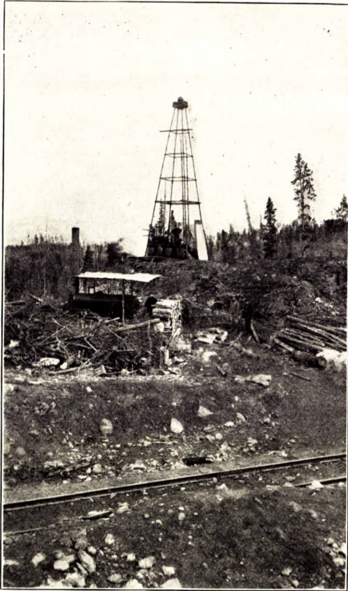
Shot drill at work on the Best Chance copper prospect, Whitehorse district, Y.T.
