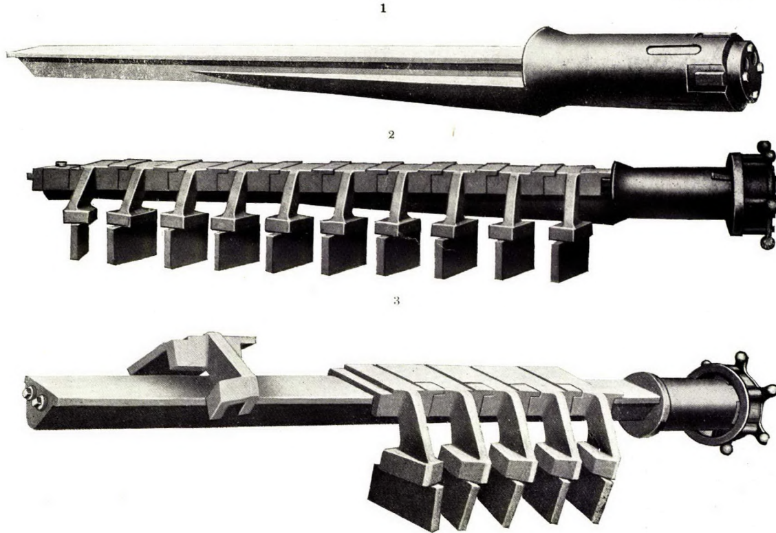
1. Rabble arm. 2. Arm dressed with rabble blade holders and blades. 3. Arm partly dressed with holders and breech block.
