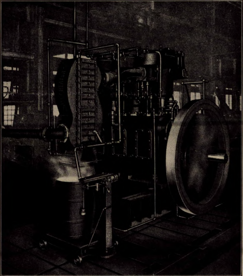
FIG. 10.—No. 8 Williams Transverse Current Water Heater, connected to Westinghouse Machine Co.'s 200 H.P. Engine.
