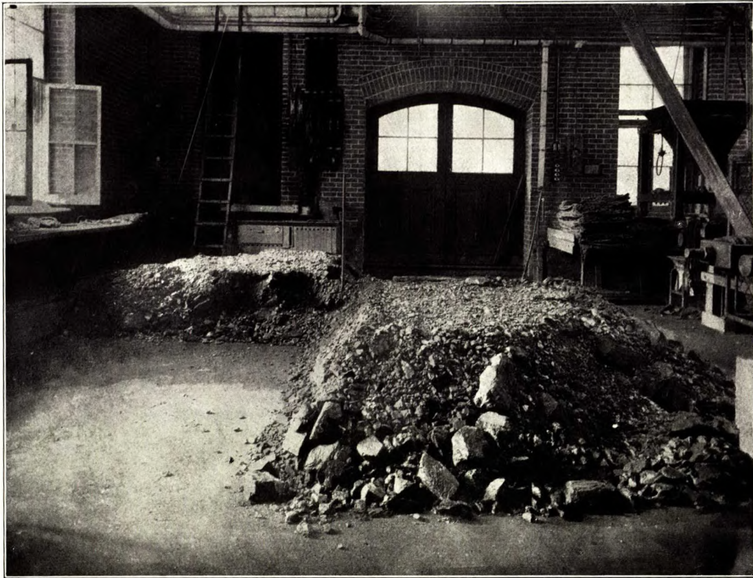
Sampling. A quartered pile of coal. Department of Mining and Ore Dressing, McGill University.
