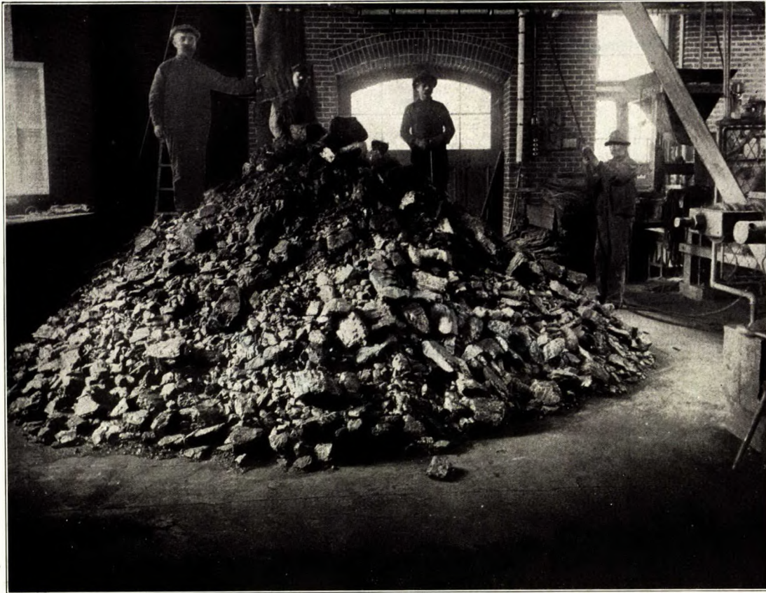
Sampling. A cone of unbroken coal. Department of Mining and Ore Dressing, McGill University.
