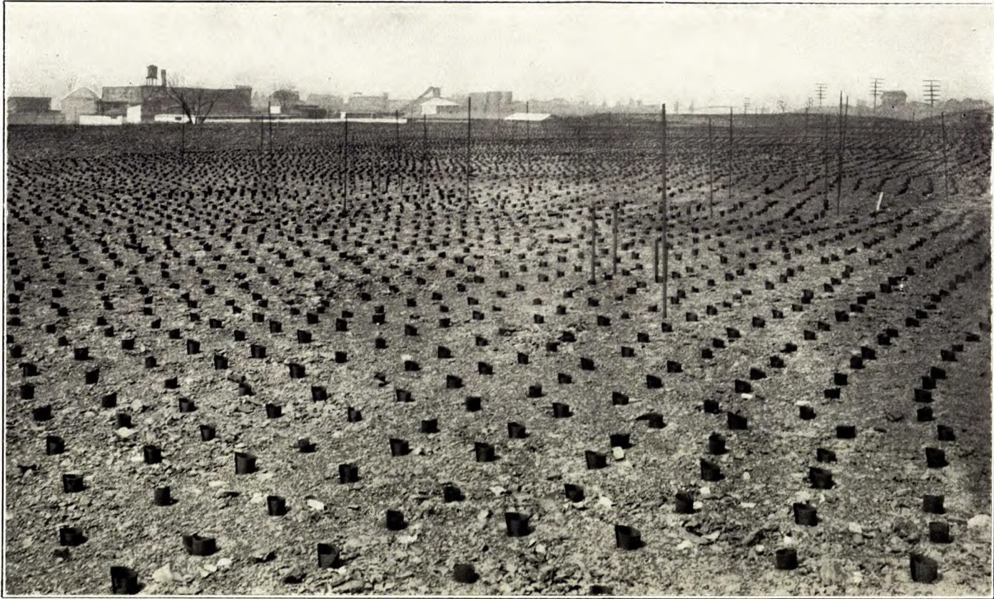
Ventilated coal pile at Montreal.
