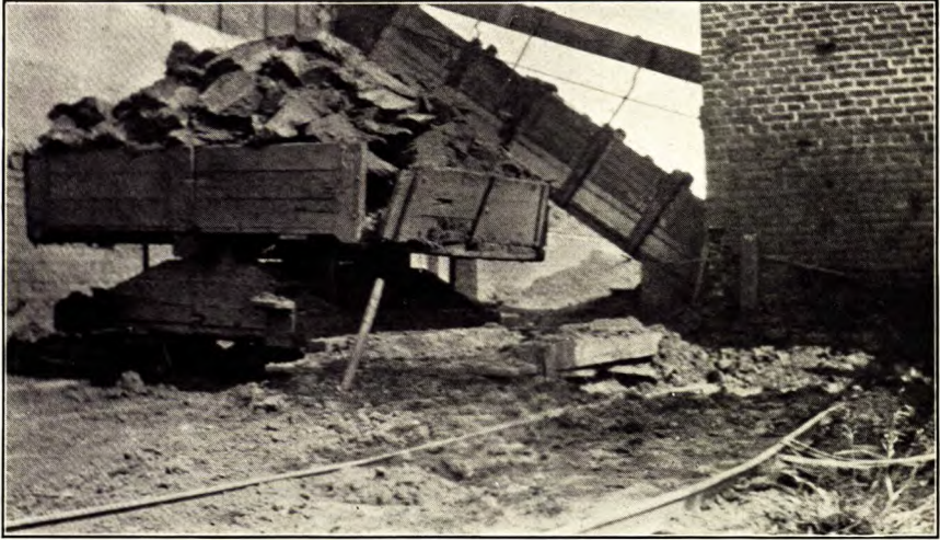
Car for Transport of Raw Peat, Ökaer, Denmark.
