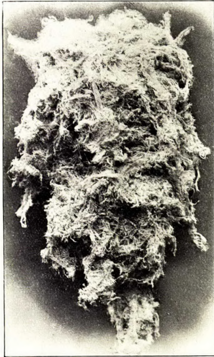
A Bunch of Fiberized Asbestos, ready for the Market.
