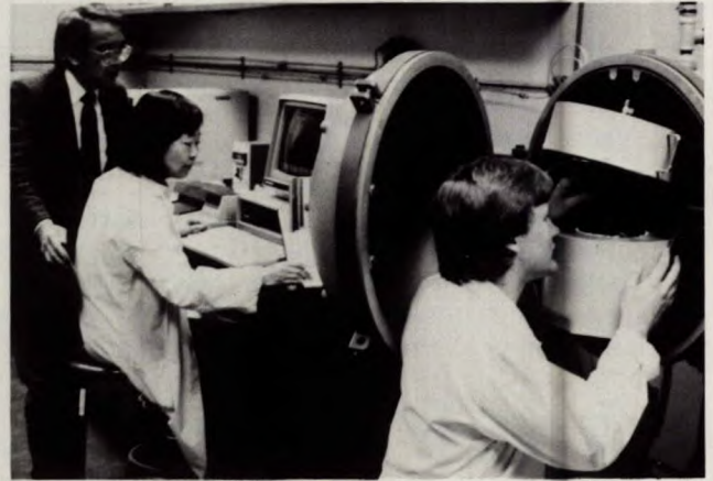
Dr. K.K. Feng (Research Scientist) operating the accelerating rate calorimeter, which is used for testing the thermal stability of explosives
