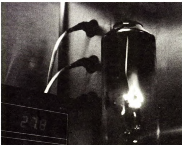
Oxygen index apparatus used in testing the flammability of conveyor belts
