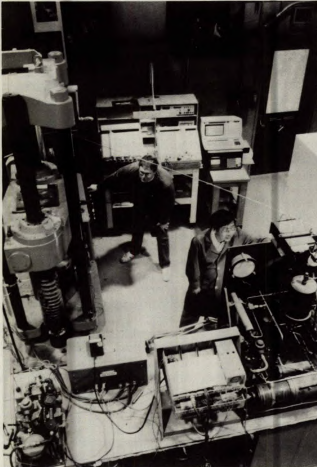
Rand Jackson and Ah-Soo Wong (Physical Scientists) conduct stiff triaxial tests on a 300 000 lb. load frame and confining pressure panel
