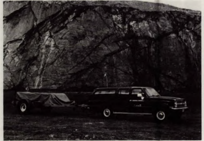
CANMET's Surface Mining Laboratory's rolling resistance trailer in the field at a western Canadian surface coal mine
