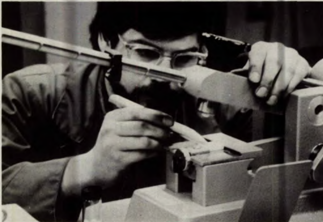
Don Cox (technologist) tests a high explosive on a BAM friction machine
