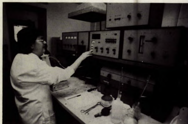
Research scientist, Elsie Donaldson, analyzing for trace elements using an atomic absorption spectrophotometer
