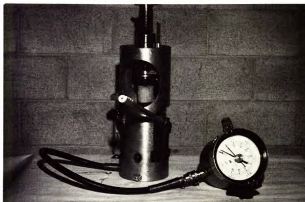
Robertson point load tester used to test rocks
