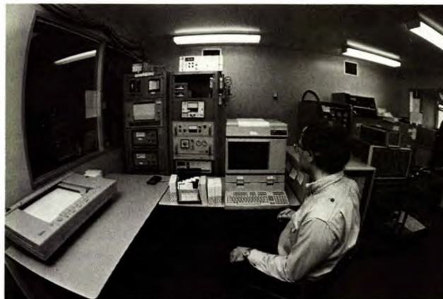
Dr. E.J. Anthony, Research Scientist, operating the computer-controlled data acquisition system and analyser bank for the pilot-scale fluid-bed combustor
