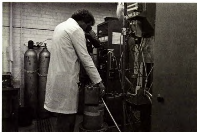
Induction furnace unit with viscosimeter attachment. G. Lemieux, Ceramic Technician, measuring viscosities of high-temperature silicate melts
