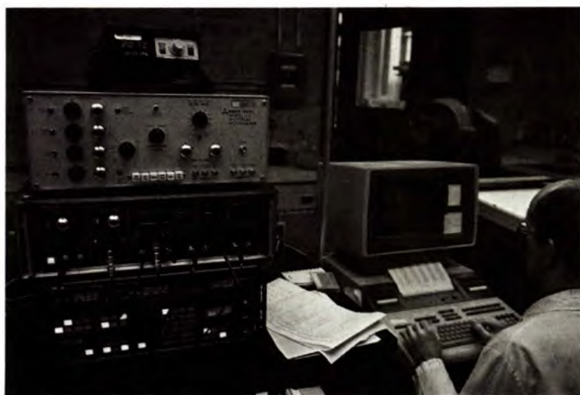
Equipment for the automated testing of electrical conductivity of ceramics. G. McDonald, Operator
