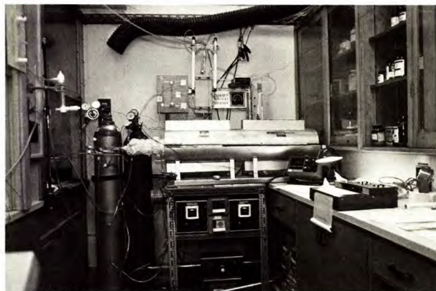
Electrochemical apparatus for the determination of thermodynamic properties of arsenides in the laboratory of Jim Skeaff, Research Scientist
