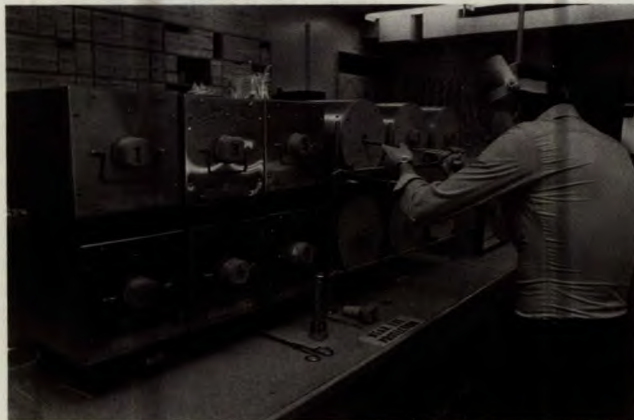
J.H.G. Laflamme, with furnaces used to synthesize compounds used as reference standards in electron beam analyses
