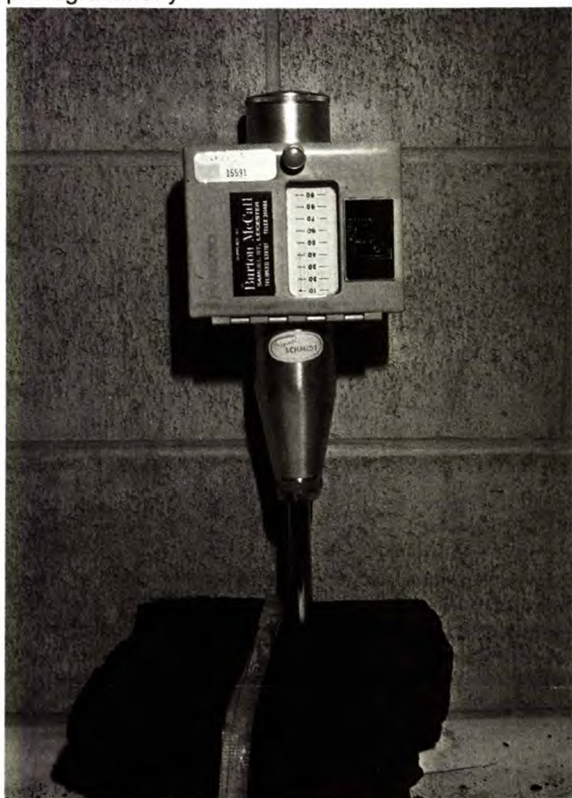
Schmidt hammer for testing rebound hardness of rock
