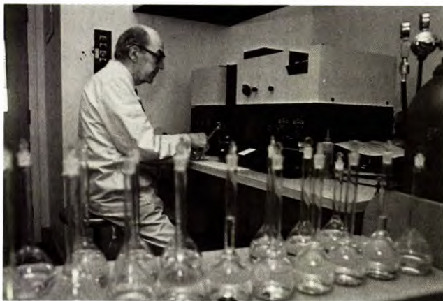
R. Craig, Chemist, analysing metal in ores with an atomic absorption spectrophotometer
