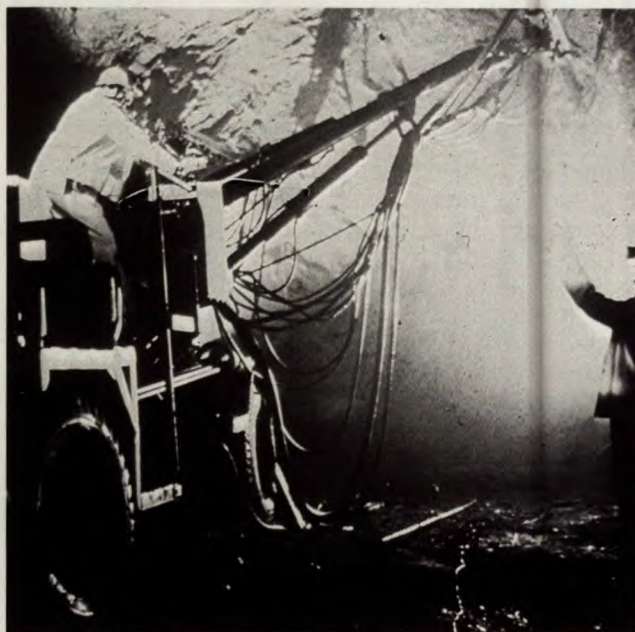
Drilling a face — a typical mining operation that can pollute the underground environment with dust, noise and vibration
