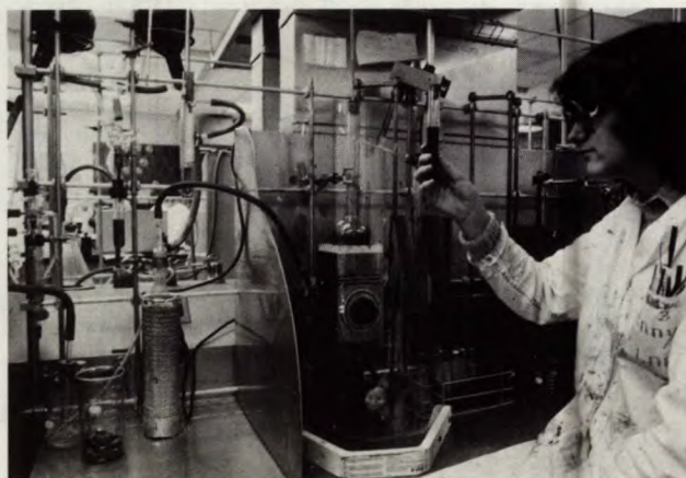
LECO sulphur analyzer used to determine sulphur levels in liquid and solid fuels
