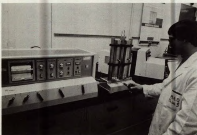
Liquid chromatograph used to operate hydrocarbon types in synthetic fuels on a preparative scale
