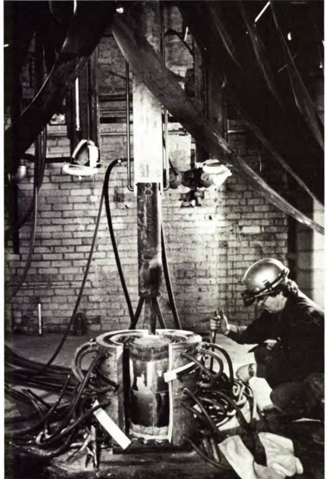
Electroslag Casting H.P. Guindon of the Foundry Section stripping a cast aluminum mould from an electroslag-cast steel shape.
