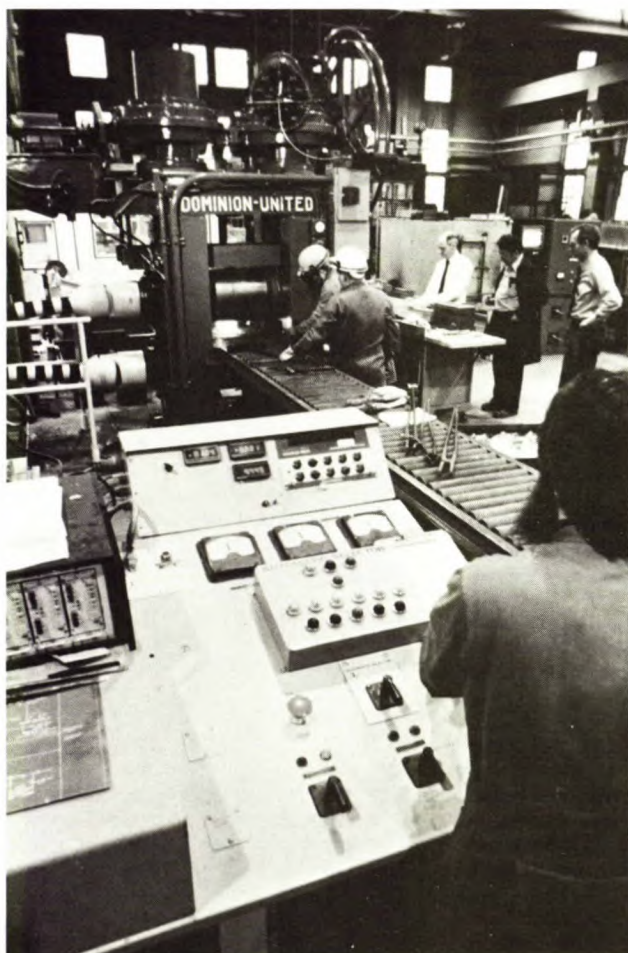
Rolling Mill Processing Technology Staff of the Metal Forming Section conducting tests on the PMRL/CAN-MET experimental rolling mill to establish rolling schedules for a thick-gauge linepipe steel.
