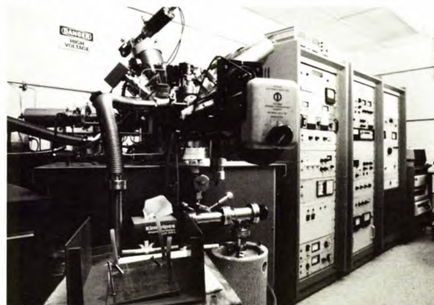
X-ray photoelectron spectrometer used in the analysis of sulphur characteristics
