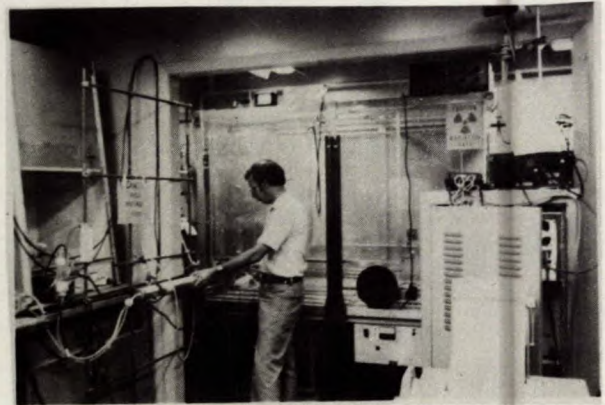
J. Bigu, scientist prepares radon box for calibration of radiation instruments
