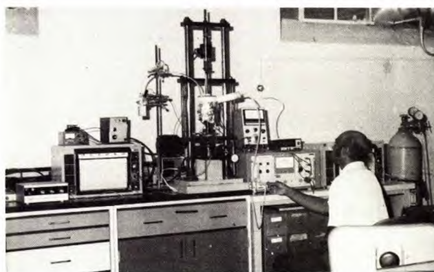
Technologist R. Ramsingh tests susceptibility of linepipe steel to stress corrosion cracking by slow strain rate technique
