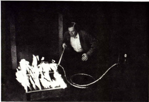
Researcher M. Ralph ignites propane burner for gallery testing conveyer belt
