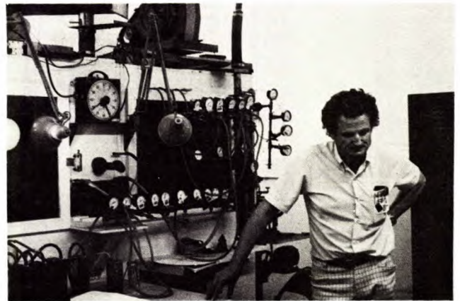
G. Knight, scientist explains the operation of the dust chamber for checking the operating characteristics of dust monitoring instruments
