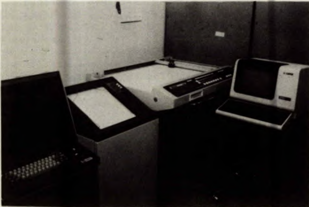
Graphics used at Mining Research Laboratories: (L to R) 4014 Tektronix terminal; Versatic 1200 hard copy device; 4663 Tektronix plotter; Digital VT131 terminal
