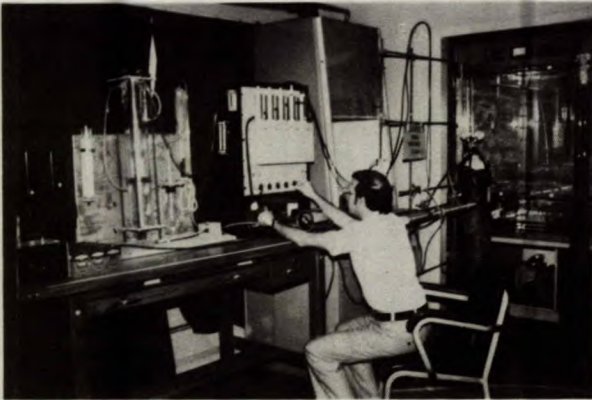
J. Bigu, scientist measures radon and thoron concentrations in uranium ore samples
