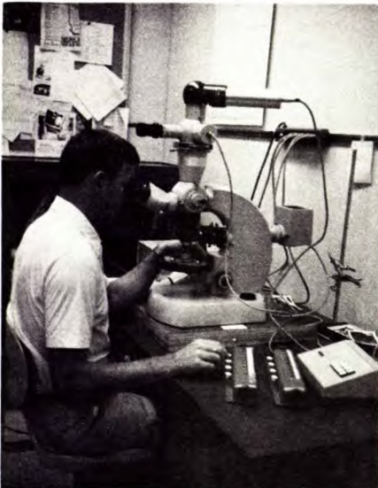
N. Ramey, technologist, uses Carl Zeiss OlK reflecting light microscope to determine textural structures in metallurgical cokes (R) for relating microscopic structures to coke quality
