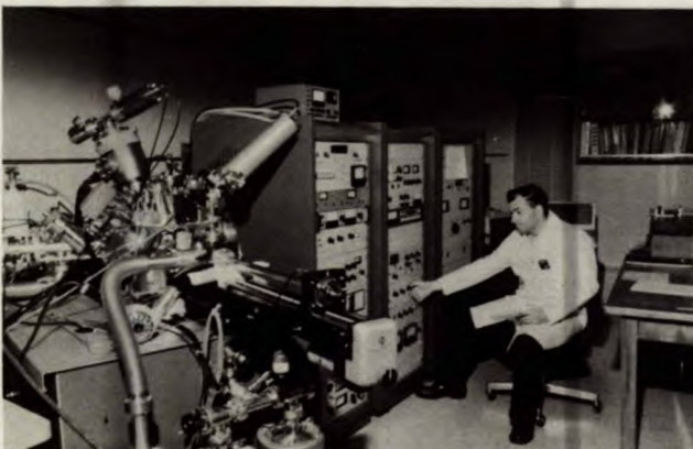
Technician L. Galbraith operates multi-technique analytical surface spectrometer having X-ray photoelectron, ultra violet photoelectron and auger electron spectroscopic capabilities - hydrotreating catalyst and coal surfaces can be analyzed for pertinent chemical information
