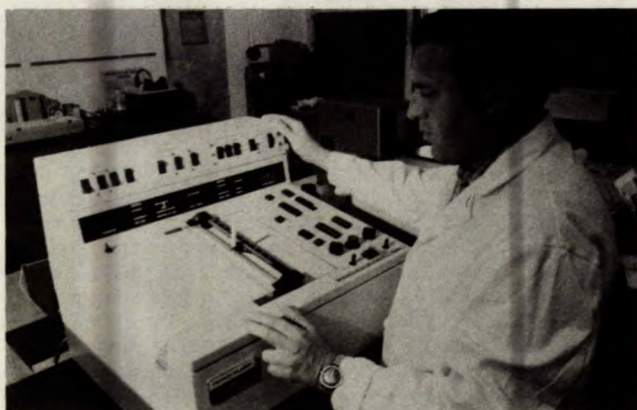
H. Barber, technician, uses infrared spectroscopy to examine a heavy oil fraction
