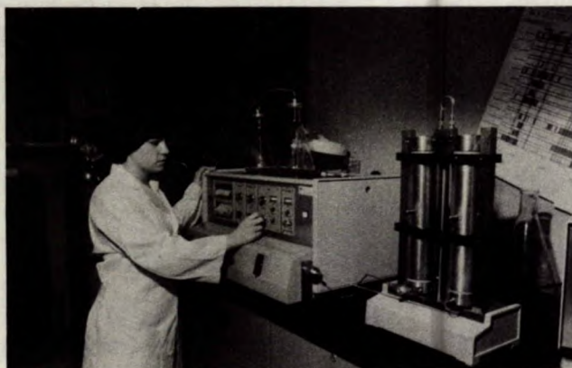
M. Curtin, cooperative student, separates heavy oil and bitumen using preparation-scale liquid chromatograph
