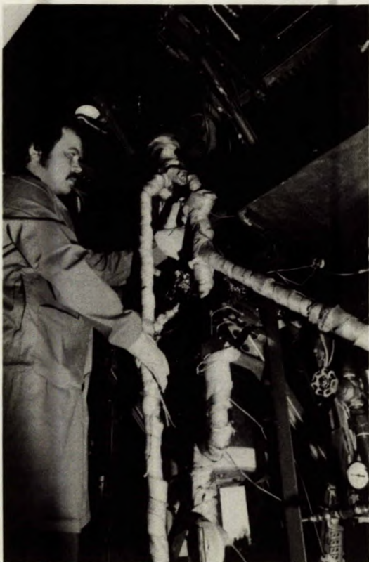
Technologist J. Whitten works on pressure vessel system of continuous flow coal liquefaction unit
