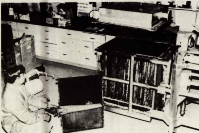
J. Vallières examines cloth of diesel exhaust filter for removing soot from engine emissions
