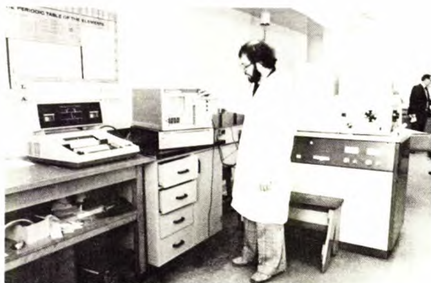
C.W. Smith, scientist performs X-ray analysis to determine thorium yttrium and rare earth elements in ores
