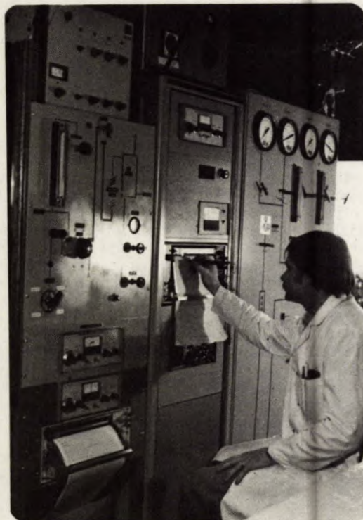
M. Fulton, technologist takes readings during an experimental run in CANMET's bench-scale catalytic hydroprocessing laboratory
