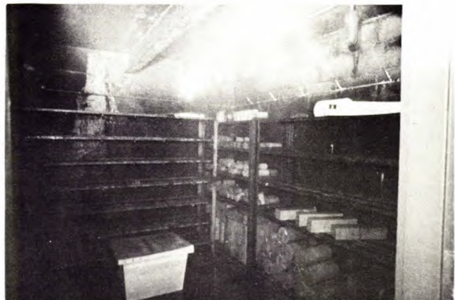
Testing concrete in simulated adverse environmental conditions
