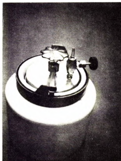
Laboratory ball mill is used in the final stage of methane desorption tests
