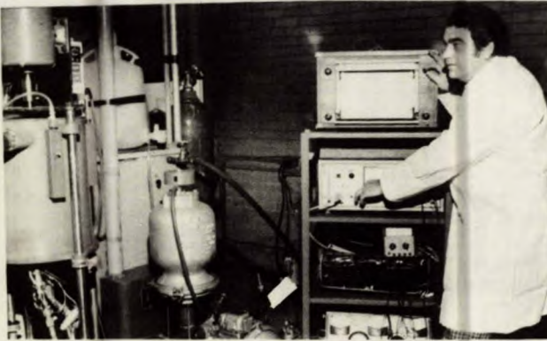
J. Bednar, technologist operates laboratory installation to test erosion/corrosion of various metals and alloys for use in coal washing plants
