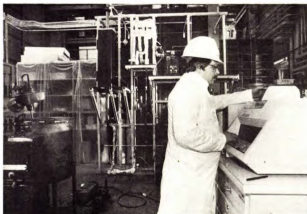
Atmospheric fixed-bed coal gasification rig in the left background with gas analyzing equipment in the right foreground
