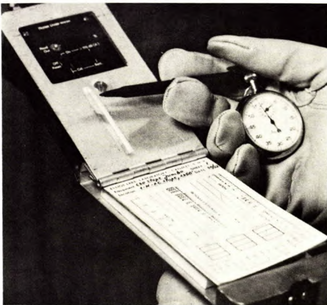
Noise monitor gun used at the Elliot Lake Laboratory to measure exposure to noise
