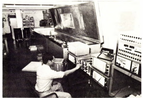
Laboratory where line-pipe samples are cyclically pressurized to determine the effect of dents, scrapes and gouges on service life
