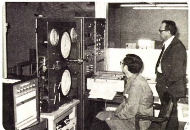
Instrumentation panel for high temperature and pressure triaxial test equipment
