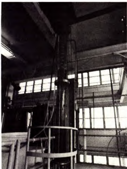
Solvent extraction column used in pilot-plant uranium processing studies in the Mineral Sciences Laboratories
