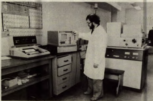
Batch samples being analyzed with the energy dispersive X-ray fluorescence analyzer
