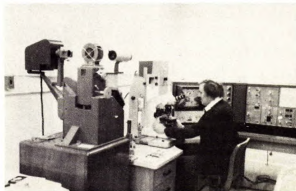
Quantimet analysis for determining size distribution of ore particles
