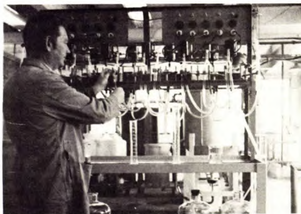
Apparatus for investigating metal recovery by solvent extraction techniques
