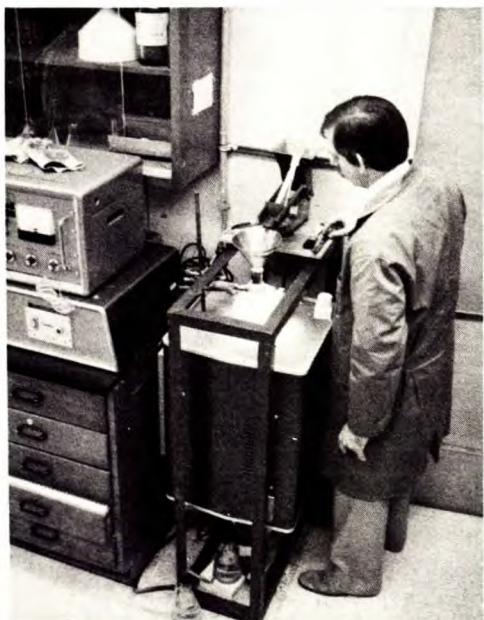
High temperature furnace for preliminary assessment of the combustible behaviour of thermal coals prior to pilot plant combustion trials
