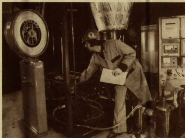
Fig. 7 - Pilot-scale fluidized-bed combustion unit; this new technique is a way of burning poor quality fuels such as low-grade coals and waste materials more efficiently and cleanly
