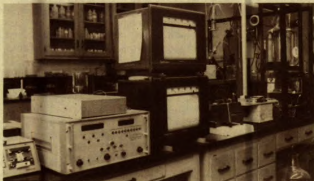
Fig. 22 - Apparatus for kinetic studies on ferric ion leaching
