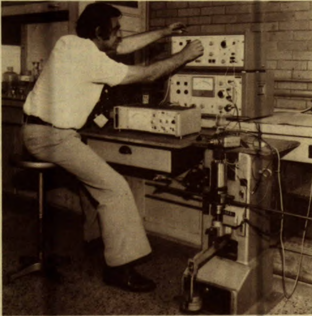
Fig. 24 - Apparatus for measuring grinding friction between steel balls over the range of electrochemical potentials
