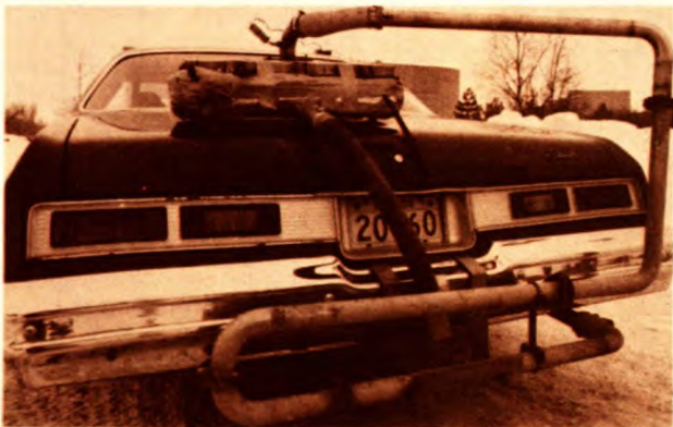
Fig. 5 - The automobile is an important user of energy as well as a major contributor to air pollution. Ways to improve fuel efficiency and reduce emissions are being studied; here lead emissions are being measured to determine the efficiency of pollution control devices.
