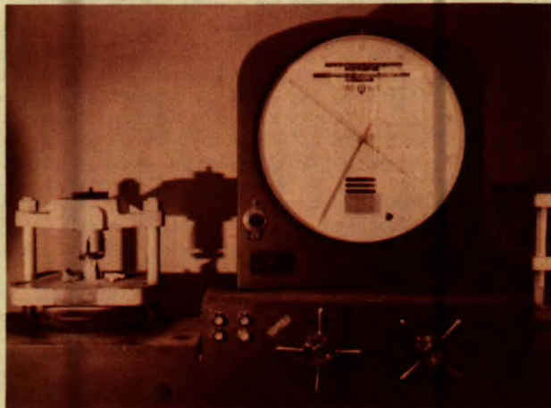
Fig. 26 - Compression test for concrete is continued to destruction of the sample to determine compressive strength
