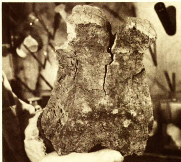
Fig. 12 - A typical piece of metallurgical coke from the CANMET oven
