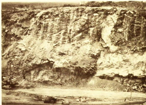
Fig. 17 - Pre-splitting — drilling and blasting a line of holes around a pit perimeter is an effective means of controlling overbreak and provides smoother, safer walls
