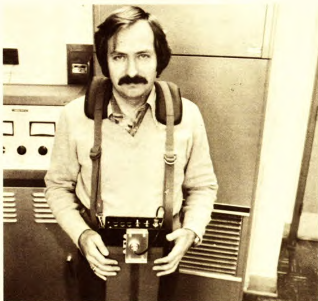
Fig. 29 - Portable radon detector developed at CANMET
