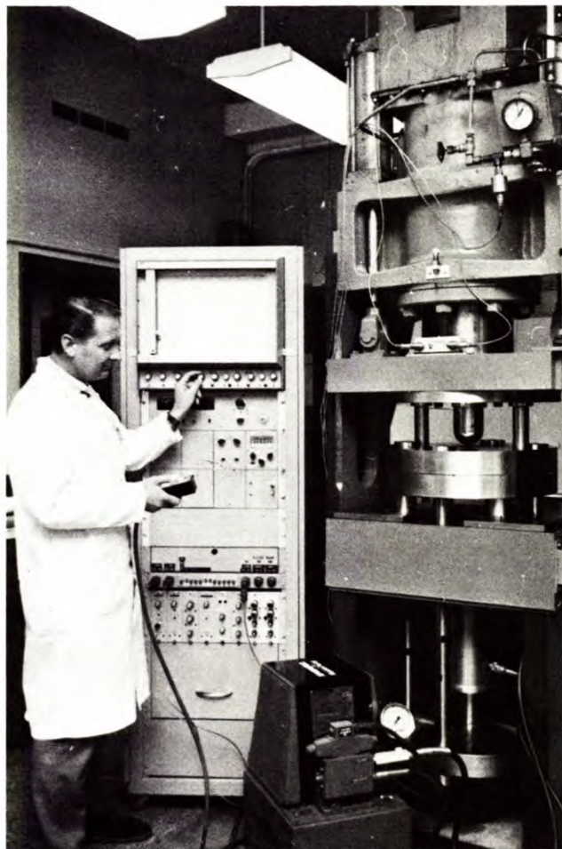
Figure 14 — A cup test is widely used to determine the formability of sheet metals. This machine is used to measure the forming characteristics of sheet aluminum or steel for possible use in automobiles.
