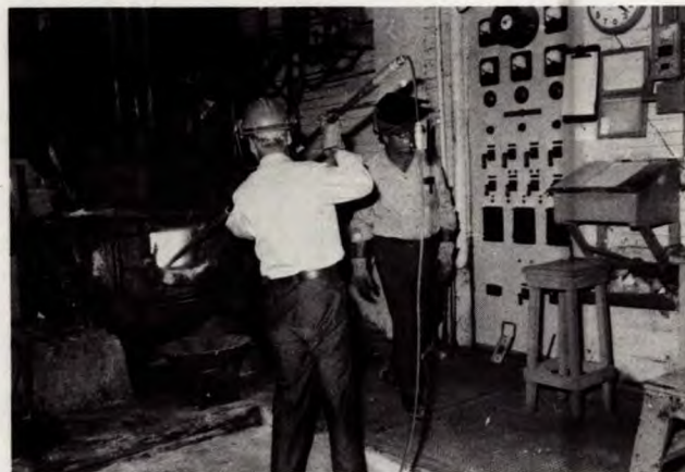
Figure 11 — The temperature of a bath of molten alloy steel is being measured in a direct arc electric furnace in the experimental foundry.
