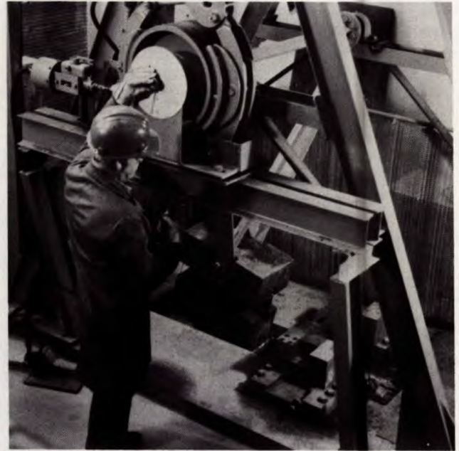
Figure 10 — The instrumented drop-weight tester is used to investigate fracture toughness of pipeline steels.
