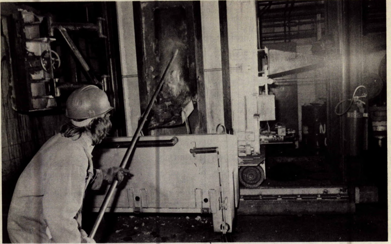
Figure 16 — Coke being removed from an oven in which coking properties of Canadian coals are tested.
