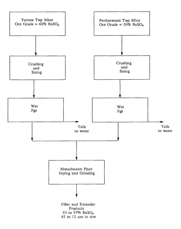
Fig. 3 - Flow diagram, Extender Minerals of Canada Ltd., Matachewan, Ont.
