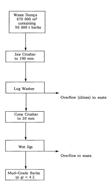
Fig. 4 – Flow diagram, Magcobar Dresser Canada, Inc., barite recovery, Walton, N.S., waste dumps
