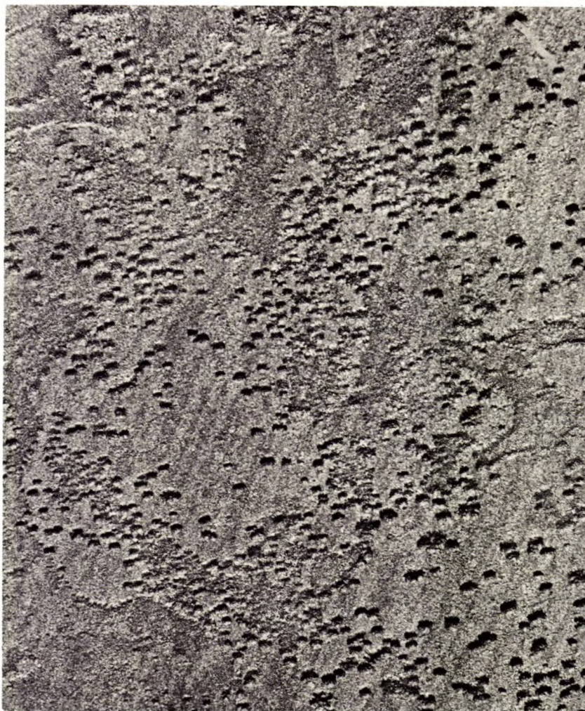
Fig. 7. Surface of specimen 2, after immersion for 107 days in Halifax Harbour, showing corrosion pits. Because of an optical illusion, these may appear either as depressions (correct) or protuberances.
