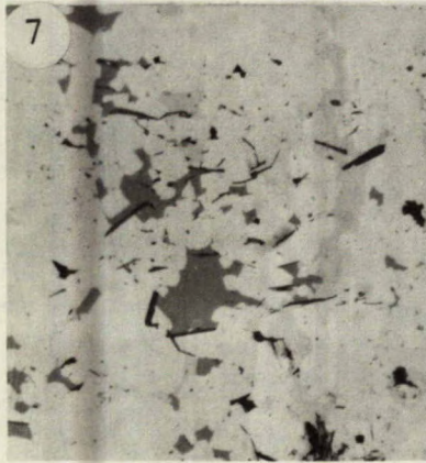
Fig. 7 - Disseminated sphalerite (grey) in massive pyrite (white)
