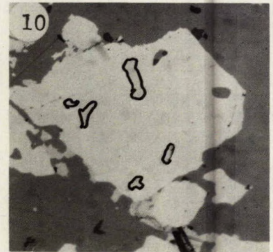
Fig. 10 - Minute galena inclusions (encircled) in pyrite. The grey is sphalerite
