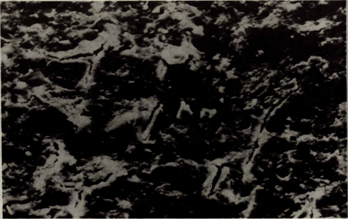
Fig. 4-5 - Surface of an epoxy-resin coating, air sprayed with a solvent (1400X) (64)
