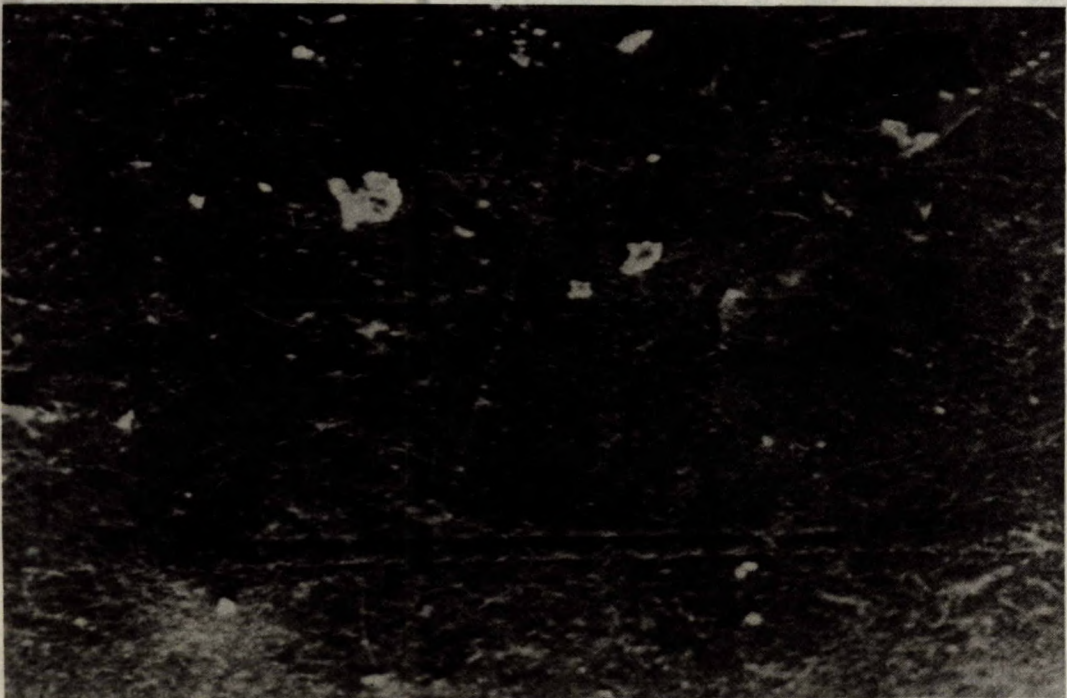
Fig. 4-6 - Surface of an epoxy-resin coating, sprayed air-free without solvent (1400X) (64)
