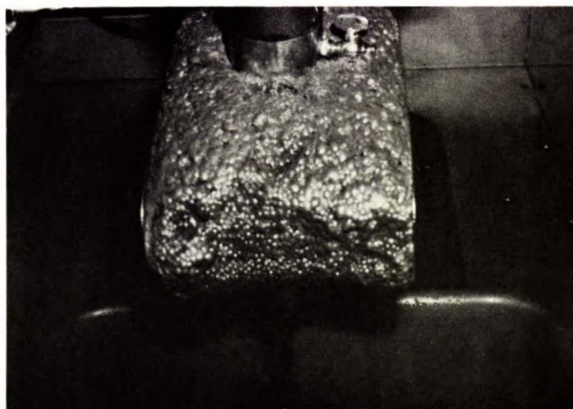
Fig. 6 - 4-L Denver batch flotation cell - zinc cleaner froth
