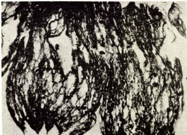
Fig. 3 - Thin sections of exfoliated vermiculite - (a) transmitted, unpolarized light X13; (b) transmitted, unpolarized light X50
