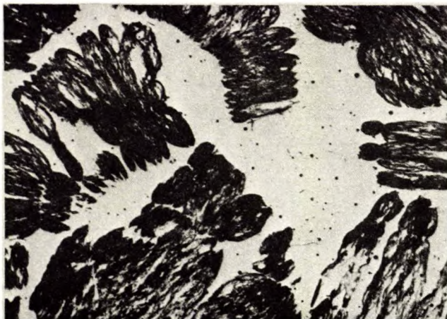
Fig. 3 - Thin sections of exfoliated vermiculite - (a) transmitted, unpolarized light X13; (b) transmitted, unpolarized light X50
