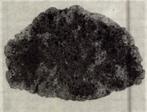
Fig. 2 - Cellular interior of bloated shale, x 4
