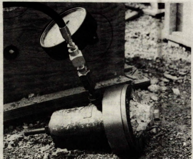
Fig. 6 - Pullout test being performed at CANMET laboratories
