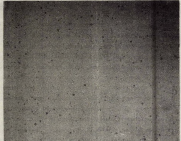
Fig. 26 - Microstructure developed in zirconia containing 7.6 mol % CaO after firing to 1550°C for 6 h
