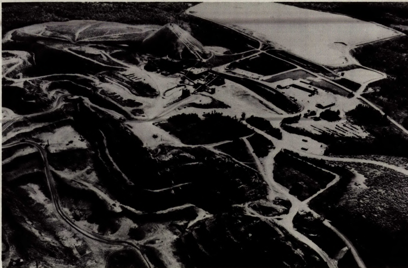
Figure 2. Open pit iron mine of Hilton Mines Ltd. near Shawville, showing waste rock dumps, upper left, and tailings pond, upper right (photo by Lister, M.&T.S., Ottawa, 1966).
