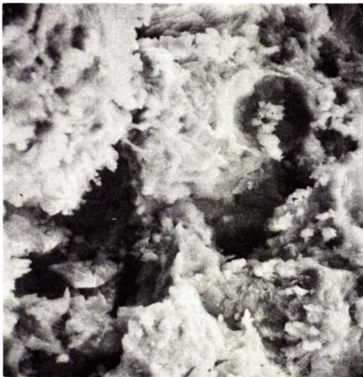
Aggregate prepared from recycled concrete x625
