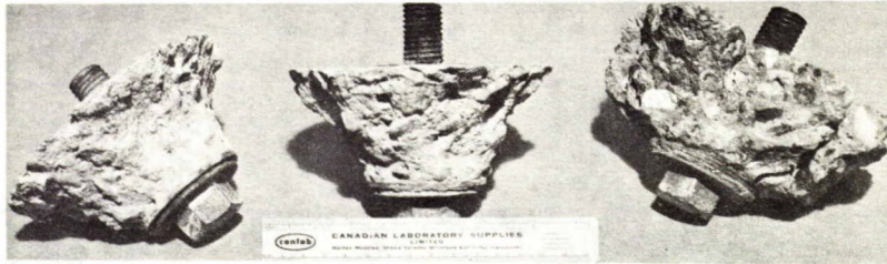
Figures 7. Pull-out assemblies with adhering cones of concrete immediately after the test.
