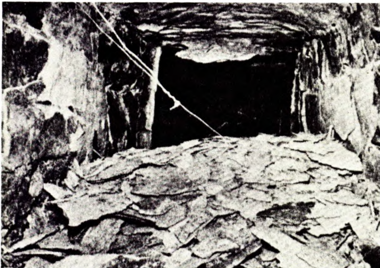
Fig. 7 - Mass of spalls in a test passage (From "Surface spalling by thermal stresses in rocks" by W.M. Gray; Proc 3rd Can Rock Mech Symp; p 85-106; Univ Toronto; Jan. 15-16, 1965, Pub. by Dept. Mines and Tech. Surveys; now EMR Canada; 1965.)
