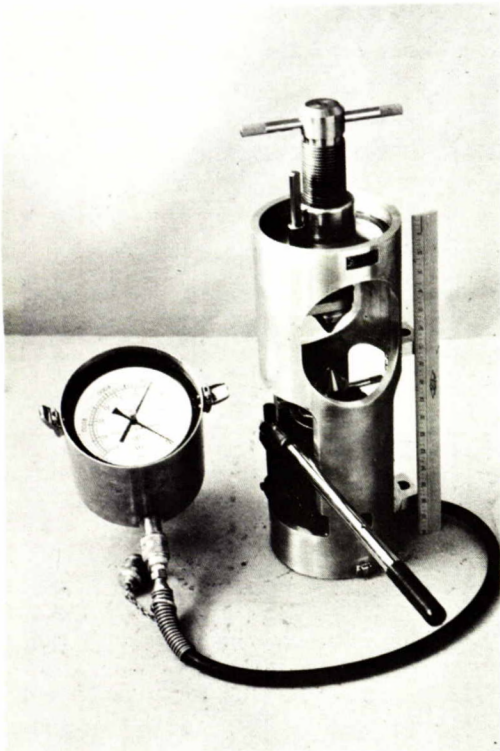
Fig 16 - Other type of point load strength testing machine (manufactured by Robertson Research Mineral Technology Limited, Wales).
