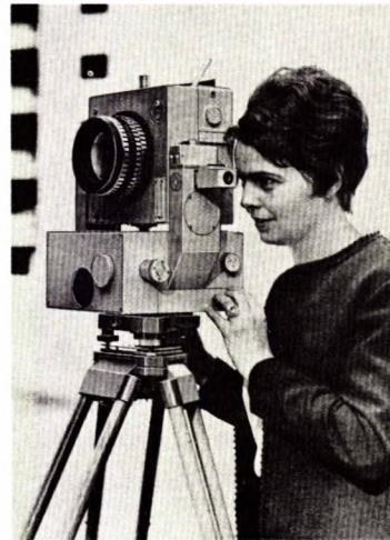
Fig 2 - 100 mm focal-length photogrammetric camera (courtesy Carl Zeiss, Jena).
