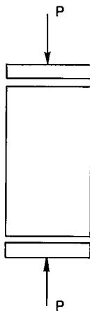
Fig 24 - Principle of uniaxial testing.
