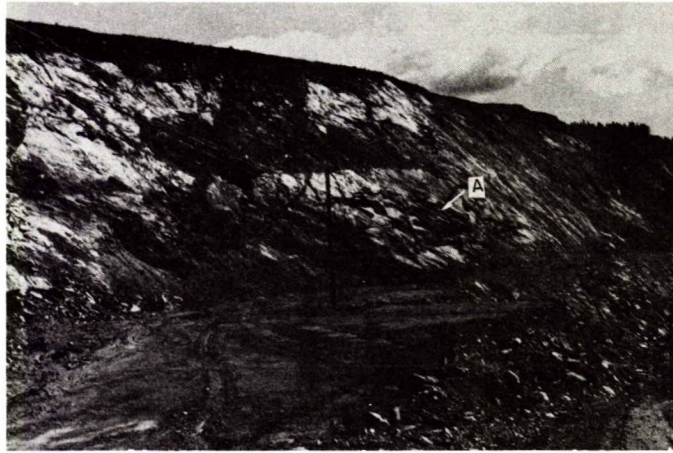
Fig 45 - View of jointing parallel to foliation (A) on north wall of Gibraltar East Pit.
