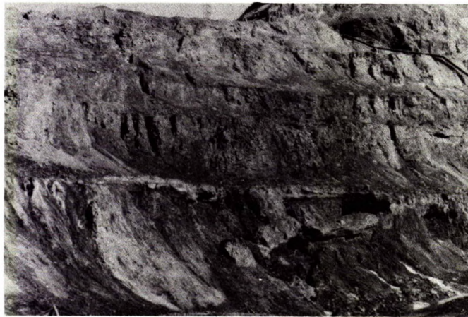
Fig 17 - Combination of rotational and plane slides; shear strength of substance and the weakness plane are the test requirements.
