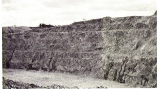
Fig. 51 - Seepage on a pit face can be observed from time to time, providing useful information on groundwater flow.
