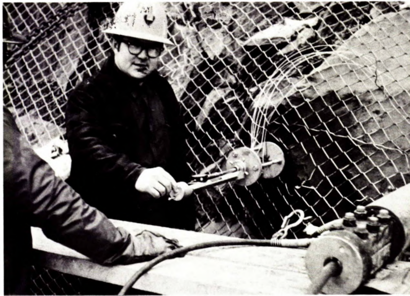
Fig E-11 - Taking measurements of a borehole extensometer.
