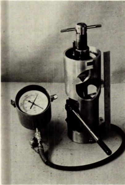
Fig 11 - Point load test machine to determine the uniaxial compressive strength of rock.
