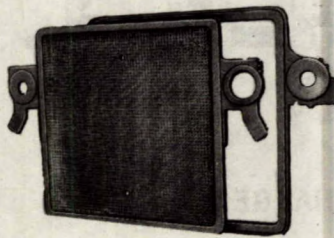
c) Side feed and closed discharge plate and frame
