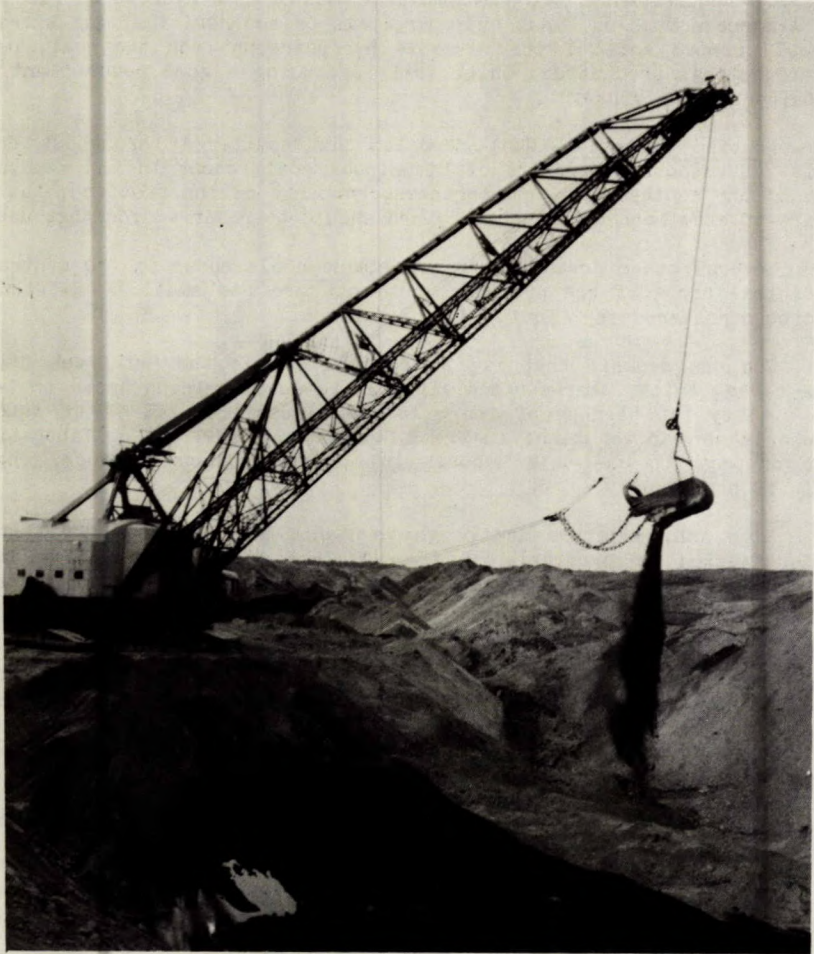
Fig. 14 - Mining subbituminous coal in Alberta; near-surface deposits such as this may be preferred over higher-grade coals because of low mining cost.
