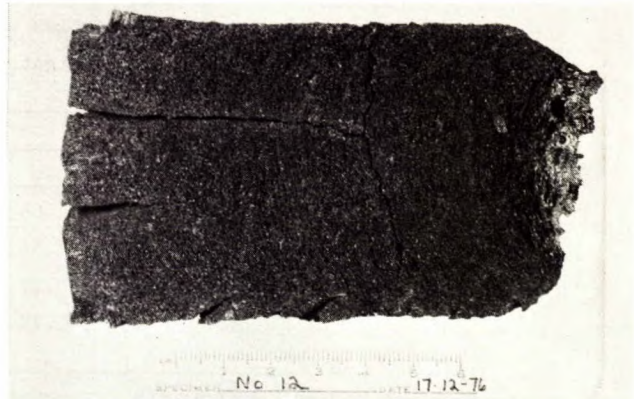
Fig. 19 - Coke section from carbonization test in which cannister was charged with coal containing 30% cylindrical briquets
