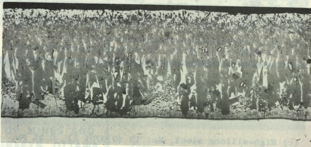
(b) High-silicon high-phosphorus steel, No. 15 (1.0% Pb, 4 minutes immersion) X300.
