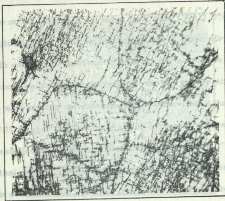
Figure 18. Fine Widmanstaetten precipitate obtained on ageing at 75°C (167°F) for 1658 days (Melt 884).
