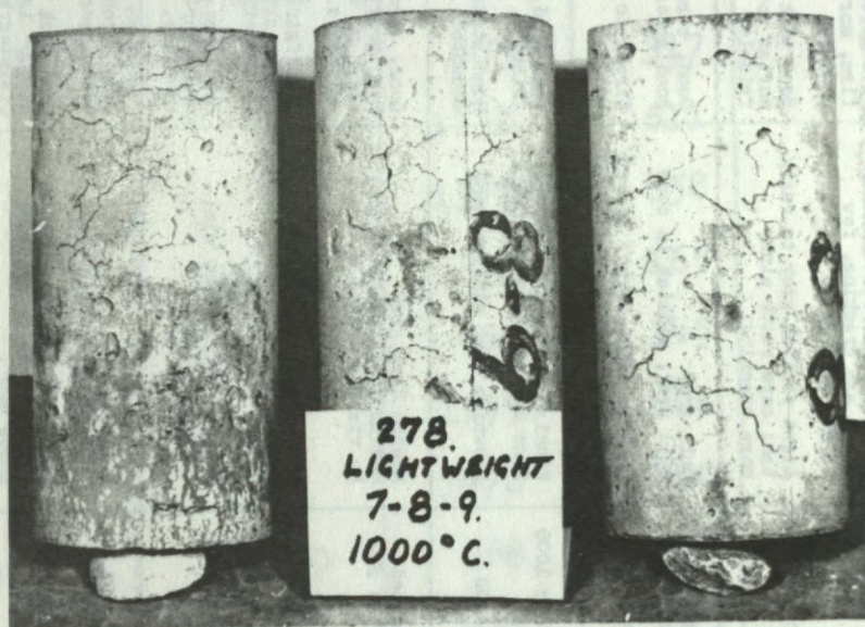
Figure 5. Expanded Shale Concrete Test Specimens Fired at 1000°C. (Note extensive surface cracking.)
